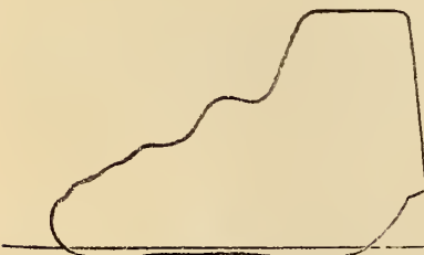
C. High-pressure—Top of Cylinder. Steam ..... 115 Vacuum ..... 18 Revolutions ..... 53
